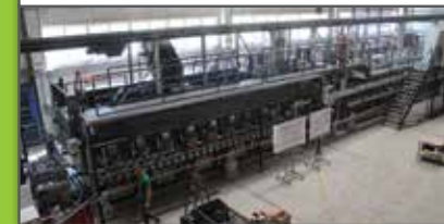
Bosio - Škoda NEW The automatic continuous roller-heat line for heat treatment of forged parts which is able to process 24 tons of forged parts per day.
